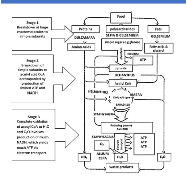
Simplified diagram of the three stages of cellular metabolism that lead from food to waste products.
